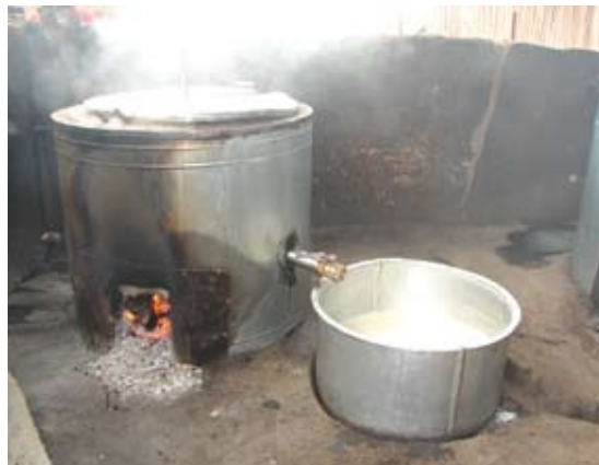
The pasteurisation facilities pasteurise around 4 000 litres of milk per day
